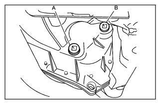
If the level is below the bottom of the filler plug hole, located on the transfer case, you'll need to add some lubricant. Add enough lubricant to raise the level to the bottom of the filler plug hole. Use care not to overtighten the plug.
